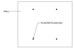
ATTACH THE MOUNTING PLATES TO THE WALL USING THE FOUR 32mm PAN HEAD 6. SCREWS. THESE ARE TO BE SCREWED INTO THE FOUR PLASTER SPEED PLUGS. DO NOT FULLY TIGHTEN YET. CONFIRM THAT THE MOUNTING PLATES ARE LEVEL BEFORE FULLY TIGHTENING.
