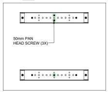
MOUNT THE MAIN FRAME ON THE MOUNTING BRACKET USING THE FOUR BLACK 8. PAN HEAD SCREWS, START WITH THE TOP TWO SCREWS, TIGHTEN ALL SCREWS TO FINGER TIGHT, CONFIRM THE RACK IS LEVEL AND TIGHTEN FULLY USING ALLEN KEY.
